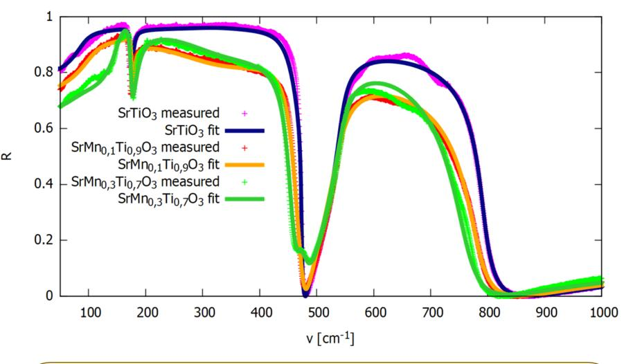
Reflectivity spectra fitted with four-parametric model of damped oscillators. Each sample has three reflectivity bands. Three TO phonons are excited at the  $\Gamma$  point for each material. In SrTi<sub>0.7</sub>Mn<sub>0.3</sub>O<sub>3</sub>, additional one phonon was observed at 186 cm<sup>-1</sup>. The soft mode frequency increases with Mn concentration and therefore the permittivity decreases with rising x.
