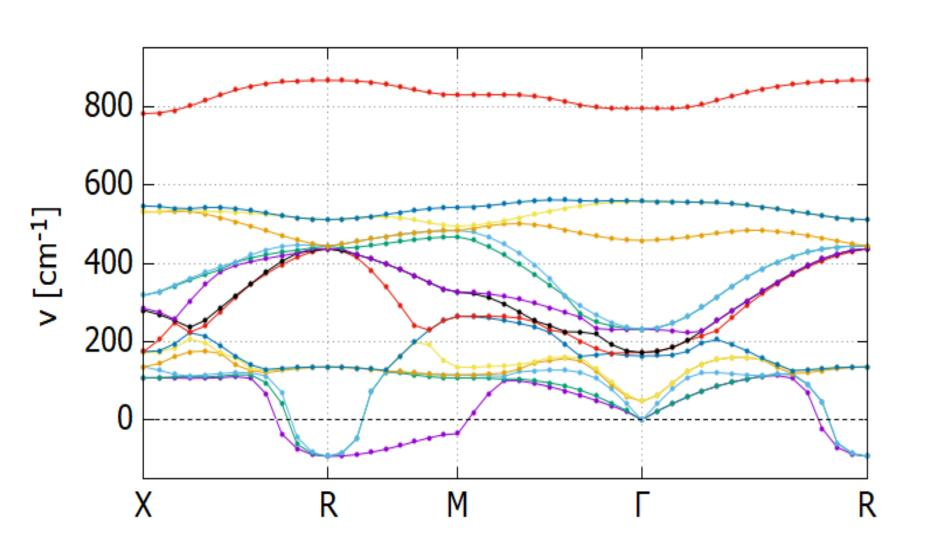
Calculated phonon spectra of STO with LO-TO splitting. Phonon softening at the R point can be seen. It is well known that this phonon softening causes structural (antiferrodistortive) phase transition at temperature 105 K from cubic to tetragonal symmetry.
