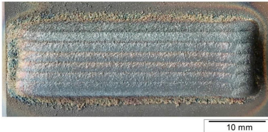
Figure 1: Laser cladded sample of the AISI H13 tool steel with five layers (top view).
