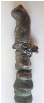
Figure 1: Result of optical floating zone growth attempt. The only successful attempt without any drop.
