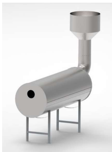
Figure 2: The final design of the collecting chamber rendered in Solid Edge 2022 software.
