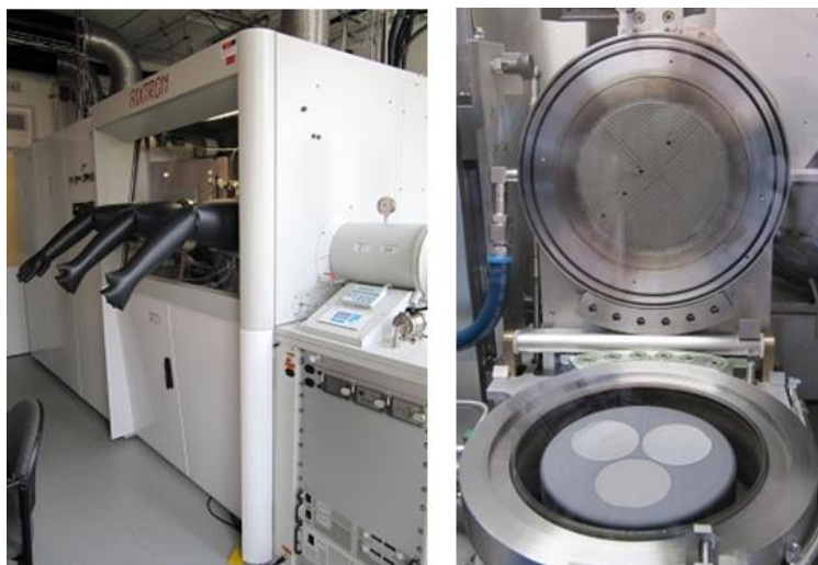
Figure 2: Glovebox for the MOVPE growth reactor and growth reactor opened.
