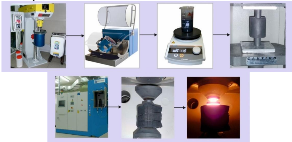
Figure 1: Scheme of creation technology of cutting ceramic sample: refinement powders (wet grinding) – evaporation – pressing – sintering [3]
