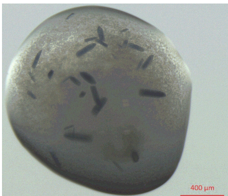
Figure 3: Crystals of MvBOxW396A, growth by the hanging drop method. Crystallization condition 0.09 M succinic acid, 14 % \frac{w}{v} PEG 3350 and protein solution 25 mM Tris/HCl, pH 7.5 with 250 mM NaCl and 25 mg · ml -1 MvBOxW396A. The line corresponds to 400 μm. (Olympus Stereomicroscope)
