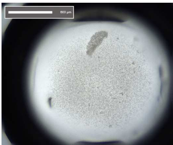
Figure 1: Thaumatin microcrystals grown by the hanging drop method. Ratio of protein solution to crystallization condition 8:10. With a crystallization condition of 20 % \frac{w}{v} NaKTart, 15 % \frac{v}{v} ethylene glycol, 0.1 M BIS-TRIS at pH 6.6 and a protein solution of 50 mg · ml -1 thaumatin and 275 mM NaAc. The line corresponds to 600 μm. (RI 1000)
